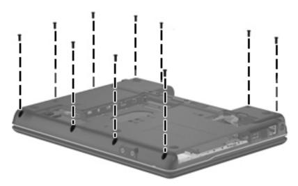
Where used: 10 screws that secure the top cover to the base enclosure
